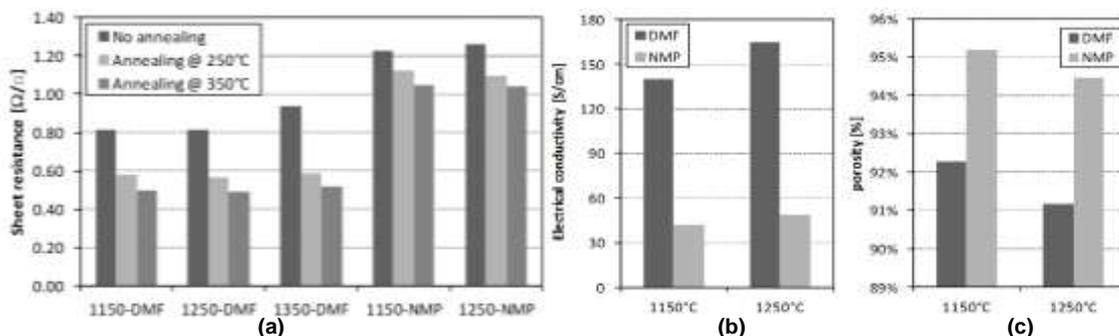
Fig. 2 – Measured sheet resistance (a), electrical conductivity (b) and porosity (c) of produced GNP thick films.
