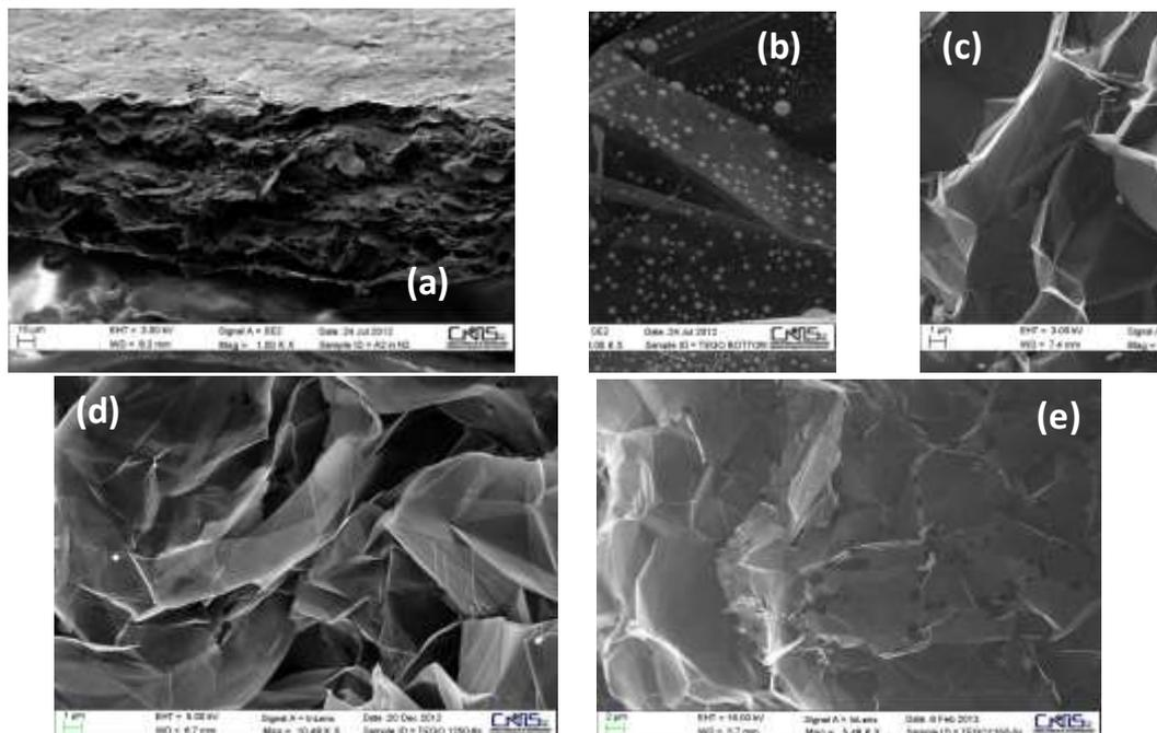
Fig.1 – SEM images of GNP thick film (a), and TEGO exfoliated at different temperatures and collected from the bottom (b) and top (c-e) of the crucible.
